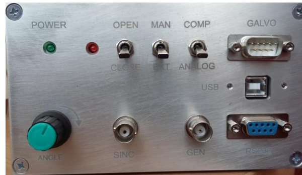
Fig. 5 Front panel of shutter controller
